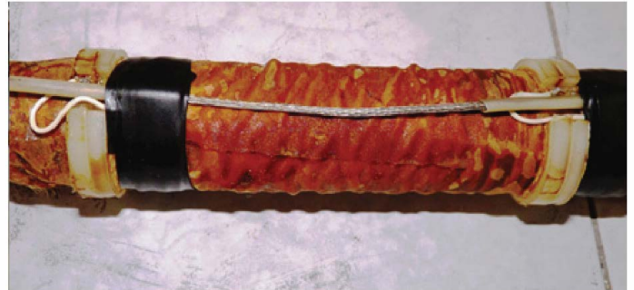
Figure 2c. The internal structure of the antennas: Each coil has about 12000 turns of wire, 0.14 mm in diameter. The exterior diameter of each coil is 31.1 mm.
