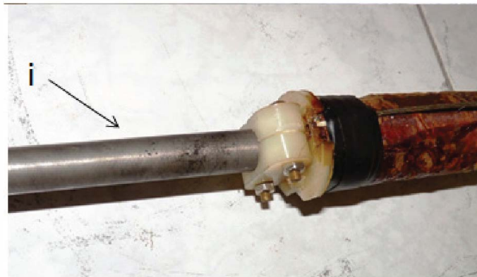
Figure 2d. The internal structure of the antennas: The core diameter (i) is 14.75 mm. The length of each coil is 113.55 mm, and the total number of coils is 1000 mm. The core length is 2000 mm.
