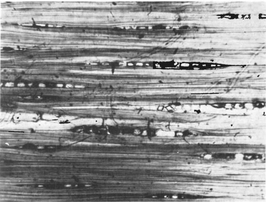
Fig. 19. Guarea Guidonia (L.) Sleumer. Tangential section \times 120 . Medullary rays of one cell in width and fibres of thick wall. Cells of medullary rays contain mastic material
