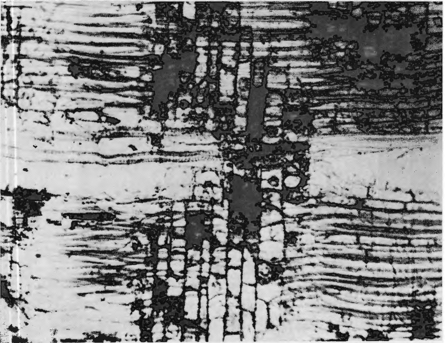
Fig. 6. Luehea speciosa Willd. Radial section \times 120 . Heterogeneous medullary rays, vessels and fibers. Cells of medullary rays contain polygonal-shaped crystals of mastic material. Marginal cells contain
