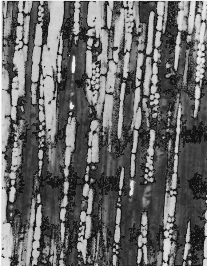
Fig. 22. Mastichodendron foetidissimum (Jacq.) Cronquist. Tangential section \times 120 . Medullary rays with 1 or 2 cells in width, fibers and longitudinal parenchyma
